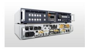
**VIO 4K (Ref. V701)** is a powerful multi-format converter offering the latest generation of digital connectivity. The product started shipping mid-February, 2016. Natively equipped with seven inputs, **VIO 4K** enables the conversion of a multitude of signals including: Dual-link DVI, DisplayPort, HDMI, 6G-SDI Optical, and Universal Analog, into an impressive array of output signal formats up to 4K 30Hz.
