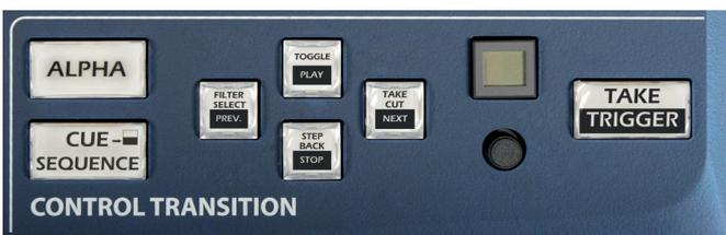
The **CUE SEQUENCE** button is used to switch the Control Transition section to **CUE SEQUENCE** mode in order to control the cue sequence playback.
