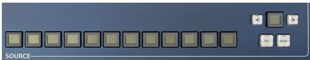
Use the left/right arrow to navigate into the source page. Then simply press the desired source in order to fill the layer(s).
