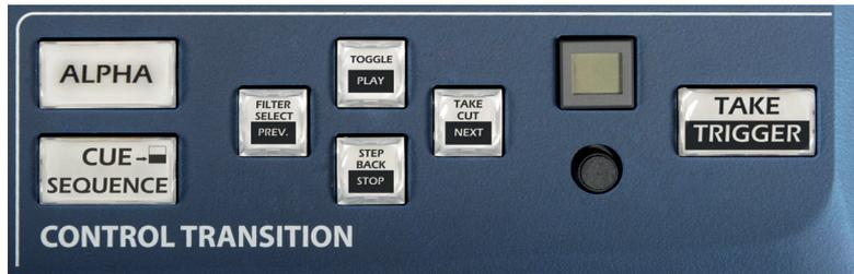
Into the control transition section, you can choose either to control the transition (default section behavior) or to control the cue sequence playback.
