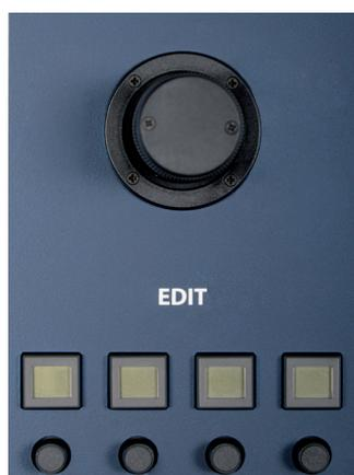
For all numerical settings, you can choose to update them roughly via the Joystick, finely via the encoders, or directly via the numpad. To enter a specific value via the numpad, press the button above the encoder to activate the numpad on the **EDITpad** and then enter the desired value. When ready, press the **ENTER** button to apply the new value.
