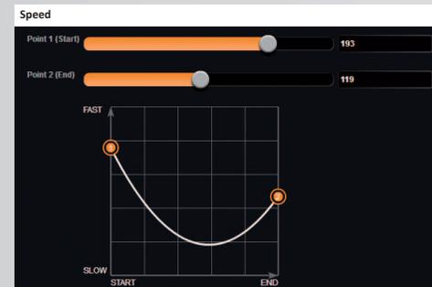
Speed: Capability to manage specific speed for each layer
